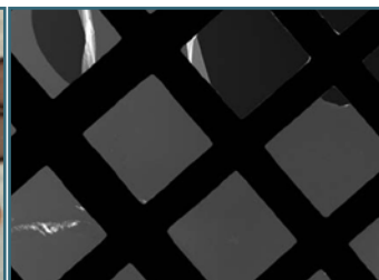
Fig. 4: Layer floated from mica onto 200 mesh TEM grids, visible cracks and wrinkles, carbon not covering the whole grid
