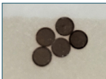
Fig. 7: Layer floated from mica onto TEM grids, neat, sturdy and dense layer
