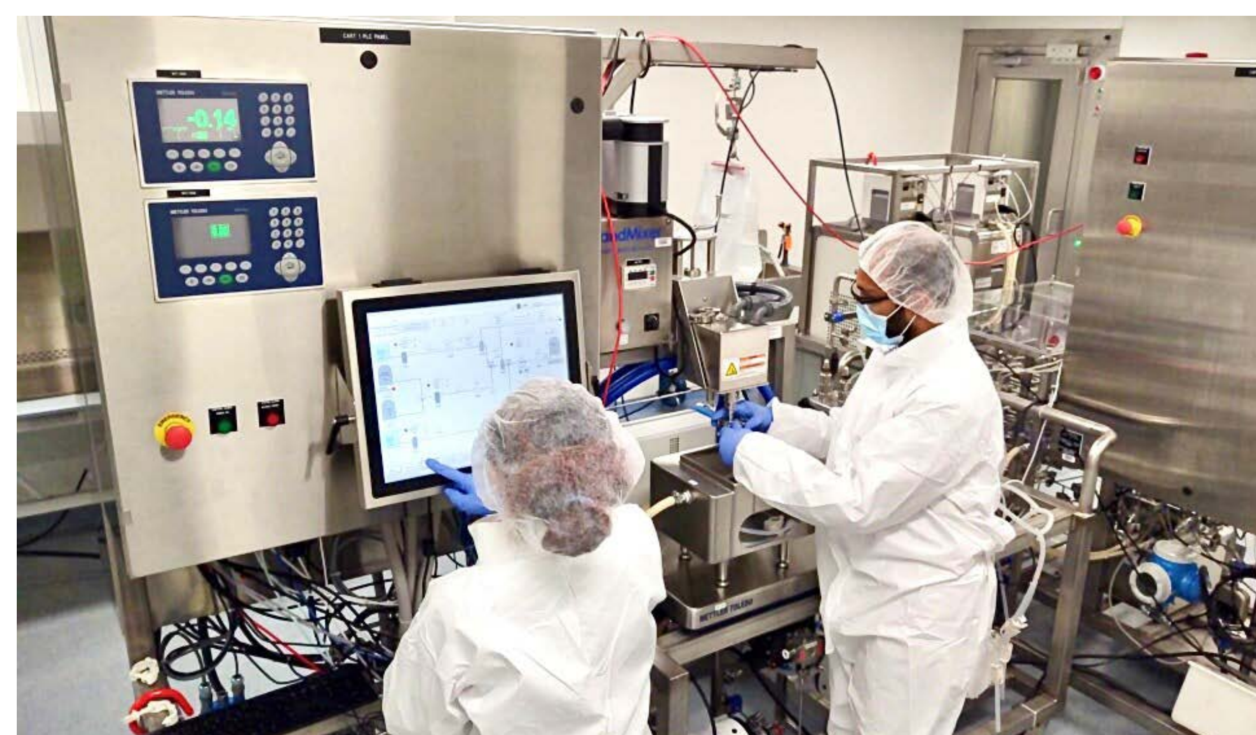
Figure 2. The UConn continuous processing skid undergoing a cleaning validation study.
