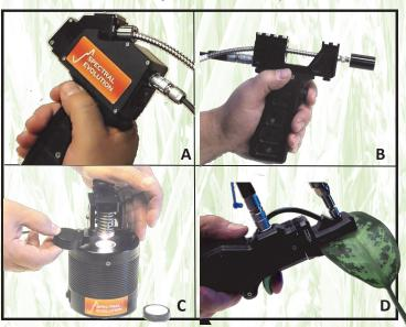
The PSR+ can also be used with fiber mount options and a range of accessories including (A) ergonomic sample contact probe with a built -in 5W halogen light source; (B) pistol grip with 1,2,3,4,5, 8 and 10° fiber mount lenses; (C) benchtop probe with sample tray and compactor; and (D) a custom leaf clip with a pushbutton trigger and an integrated light source. An integral swing-away reflectance panel provides easy reference measurements.
