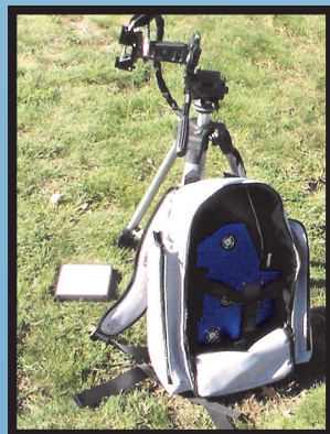
The SR-6500 fits in a backpack with two Li-ion batteries for field use.
