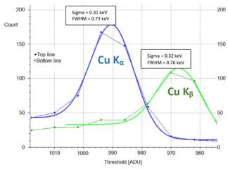
This spectrum was measured with 0.3 mm thick Si sensor performing threshold scan in frame mode.
