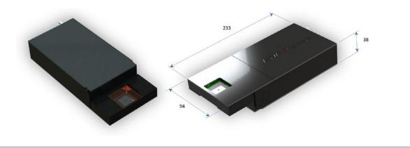
The #AdvaPIX TPX3 Quad presents a new line of ADVACAM detectors optimized for #XRD, #SAXS or similar tasks where a primary pencil beam of radiation passes through the detector without interaction. For this purpose we developed a Quad detector with monolithic sensor with central hole (the device version without central hole exists as well).
