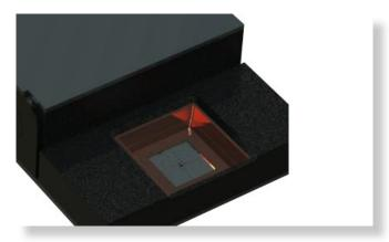
The detector design is vacuum compatible. It can be optionally connected to water cooling circuit for better temperature stabilization.
