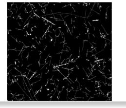
Illustration of single particle sensitivity of Timepix3 device. The tracks of different particles of radiation background (mostly muons and few protons) were recorded in 5 minutes on board of airplane. No noise (clean zero) is seen in dark regions.
