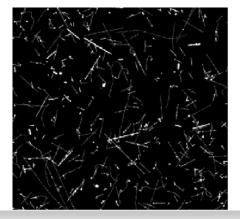
Illustration of single particle sensitivity of Timepix3 device. The tracks of different particles of radiation background (mostly muons and few protons) were recorded in 5 minutes on board of airplane. No noise (clean zero) is seen in dark regions.
