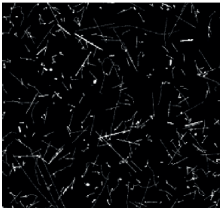
Illustration of single particle sensitivity of Timepix3 device. The tracks of different particles of radiation background (mostly muons and few protons) were recorded in 5 minutes on board of airplane. No noise (clean zero) is seen in dark regions.
