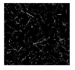
Illustration of single particle sensitivity of Timepix2 detector. The tracks of different particles of radiation background (mostly muons and few protons) were recorded in 5 minutes on board of an airplane. No noise (clean zero) is seen in the dark regions.
