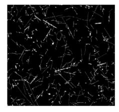
Illustration of single particle sensitivity of Timepix2 device. The tracks of different particles of radiation background (mostly muons and few protons) were recorded in 5 minutes on board of airplane. No noise (clean zero) is seen in dark regions.
