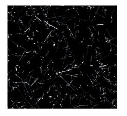
Illustration of single particle sensitivity of Timepix2 device. The tracks of different particles of radiation background (mostly muons and few protons) were recorded in 5 minutes on board of airplane. No noise (clean zero) is seen in dark regions.
