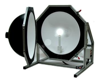
The B-IS500 integrating sphere ensures the accurate measurement of total spectral radiant flux of compact light sources.
