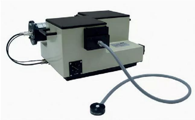
The B-TanTest150 solution provides users with an accurate and reliable solution used to accurately quantify the UV emission of a given source in accordance with IEC 60335-2-27 2010.
