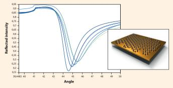
Single monolayer of graphene was measured as 3.7 Å thick at 670 nm wavelength. Thin layers form a single peak in a MP-SPR scan.
