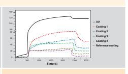
Measure interactions in real-time: adsorbed protein mass, release kinetics, swelling, etc. Here, a protein-resistant coating is evaluated.
