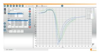
LayerSolver™ is a dedicated software module that allows fitting of multiple nanolayers simultaneously from multiwavelength measurements.
