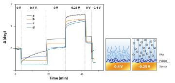
PAA polymer brushes swelling and collapse caused by pH and electric potential change.
