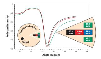
Even subnanometer differences in the inner and outer circles within a CVD chamber can be measured using MP-SPR. Here, MP-SPR discovered a 10 nm difference in metal deposition thickness towards center and 0.2 nm difference along the outer circle.
