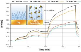
Real-time swelling of nanocellulose under different water vapour concentrations.
