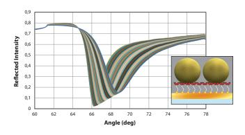
Binding of functionalized gold nanoparticles (50 nm in diameter) onto a self-assembled polymer surface measured with MP-SPR at 785 nm.
