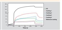
Measure interactions in real-time: adsorbed protein mass, release kinetics, swelling, etc. Here, a protein-resistant coating is evaluated.
