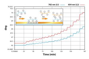
Self-assembly of polyelectrolyte multilayers is measured in real-time at two wavelengths (670 nm and 785 nm). Twenty layers are formed *in-situ*. Thickness for each layer can be determined. The true layer thickness is 2.5 nm per bilayer.
