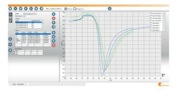
$Layer Solver^m is a dedicated software module that allows fitting of multiple nanolayers simultaneously from multiwavelength measurements.\\$
