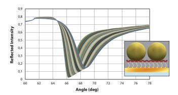
Binding of functionalized gold nanoparticles (50 nm in diameter) onto a self-assembled polymer surface measured with MP-SPR at 785 nm.
