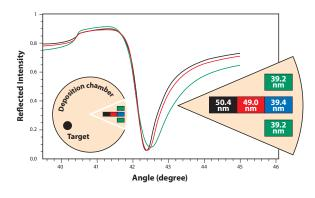
Even subnanometer differences in the inner and outer circles within a CVD chamber can be measured using MP-SPR. Here, MP-SPR discovered a 10 nm difference in metal deposition thickness towards center and 0.2 nm difference along the outer circle.
