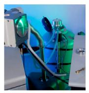
has a dovetail fitting to accept a cryo shuttle and specimen and can be precisely controlled over a temperature range from 100 °C to -190 °C or lower. Large gas cooled cold traps located above and below the specimen stage ensure clean, high vacuum conditions in the chamber.
