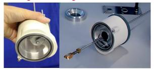
The vacuum transfer device is compact, reliably vacuum tight and has a convenient bayonet connection to the specimen shuttle to ensure rapid pick up and transfer. Set into the Prepdek<sup>™</sup> work surface is a pumped storage tube for the cryo transfer device (see Prepdek<sup>™</sup> workstation section below).
