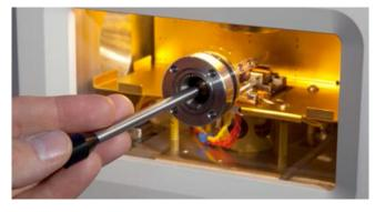
Twin fracturing tools (actively cooled) are available and allow a range of specimen types to be cold fractured.
