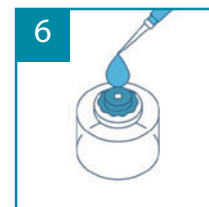
Draw up liquid sample onto the center of the chip (5 \mu l at a time).
