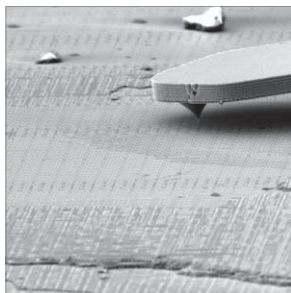
(Figure 1) SEM image of CPU chip with cantilever tip positioned on the region of interest.
