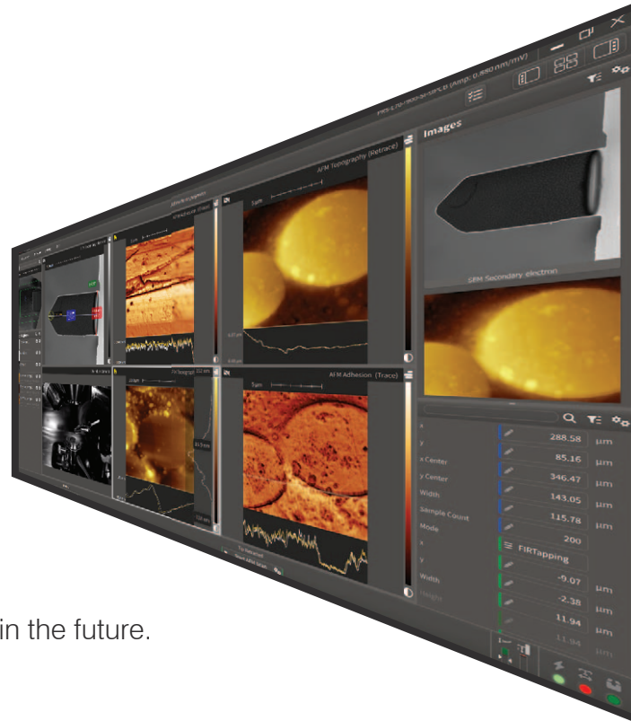
Correlated AFM and MFM data of a multilayer Pt/Co/Ta sample.
