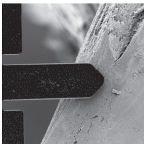
(Figure 1) SEM image of bone surface with cantilever.
