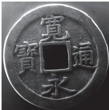
Acceleration voltage: 15 kV Image signal: SE Magnification: 30x Field of view 10 vertically × 12 horizontally (some parts were trimmed) Sample: Japanese ancient coin
