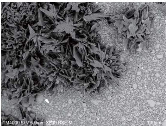
TM4000 5kV 5.9mm X1.00 BSE M Accelerating voltage: 5 kV Image signal: BSE Magnification: 500x Sample: Chocolate Cooling stage used
