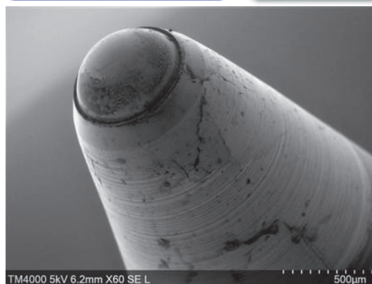
TM4000 5kV 6.2mm X60 SE L 500µm Accelerating voltage: 5 kV Image signal: SE Magnification: 60x Sample: Tip of a ball-point pen
