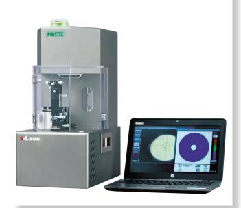
The benchtop single crystal orientation system impresses with its unique design. Compared to conventional single-crystal orientation systems, which consist of an X-ray generator, a cooling system, a Laue camera, a sample table and a safety housing, it combines all of these components in one unit.
