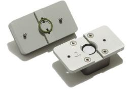
The Humidity Module is an optional module compatible with both the QSense Explorer and Analyzer systems. The module has a GORE™ membrane that separates a small air pocket above the sensor crystal from a flow system for liquid. By using different saturated salt solutions above the membrane, the relative humidity in the air above the sensor can rapidly be changed and controlled without using other equipment.
