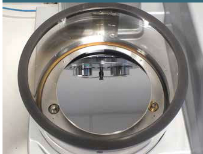
Q300T T Plus has a 200 mm wafer capability
