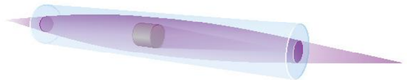
Sigray Twin Paraboloidal X-ray Mirror Lens: Illustration of the point-to-point focusing of a Sigray optic with two opposing paraboloids. The first paraboloid collimates a diverging beam, and the second paraboloid focuses the collimated beam onto a tight, achromatic focal spot.
