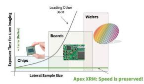
**Comparison of Apex-XCT and Leading Other 3D X-ray Microscope:** Apex XCT achieves high resolution imaging at fast throughputs that are independent of sample size (see green flat line), while other 3D x-ray approaches get exponentially slower for larger samples and thus require cutting down the sample.
