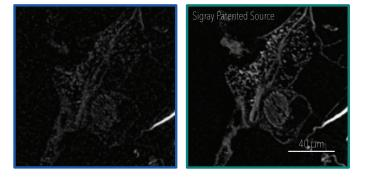
Color Imaging: By tuning the x-ray energy, the Sigray ChromaXRM can provide orders of magnitude improvement in contrast and visibility for challenging samples. Shown above are the same sample imaged under different conditions: one mimicking the best achievable contrast on the next-best XRM system available and one with the Sigray patented x-ray source.
