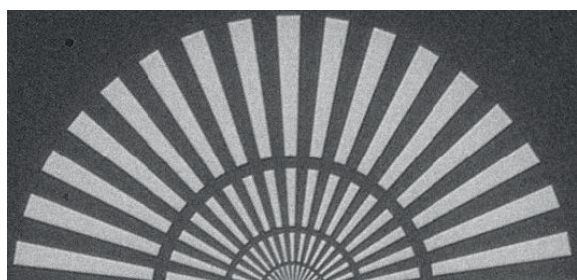
Figure 9: Spatial resolution on the EclipseXRM is 300nm (inner spoke on target is 200nm). This is almost half that of the leading x-ray microscope competitor and results in finding defects (cracks, voids) and features that would otherwise be invisible.
