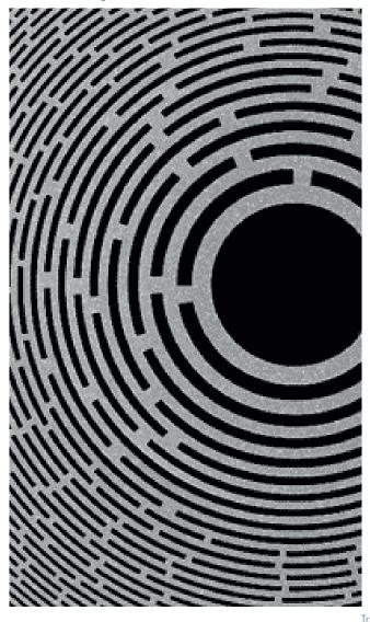
Lambda is zoneplate-based to achieve unprecedented resolutions High resolution mode: 40 nm spatial resolution | 10 nm voxel Large field of view mode: 120 nm spatial | 40 nm voxel
