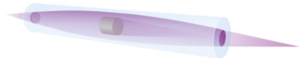
Twin paraboloidal X-ray mirror lens: Illustration of the point-to-point focusing of a Sigray optic with two opposing paraboloids. The first paraboloid collimates a diverging beam, and the second paraboloid focuses the collimated beam onto a tight, achromatic focal spot.
