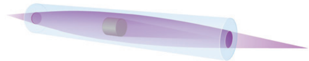
Twin paraboloidal X-ray mirror lens: Illustration of the point-to-point focusing of a Sigray optic with two opposing paraboloids. The first paraboloid collimates a diverging beam, and the second paraboloid focuses the collimated beam onto a tight, achromatic focal spot.
