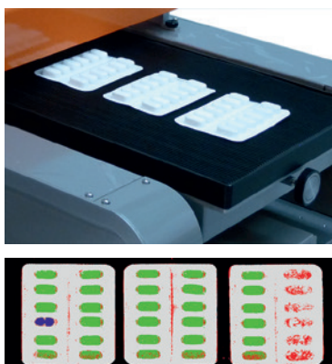
Blister package inspection. Red indicates empty blister, Green indicates normal blister and Blue indicates false product.
