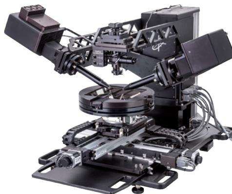
The dual rotating compensator ellipsometers RC2 are a new generation of advanced spectroscopic ellipsometry.
