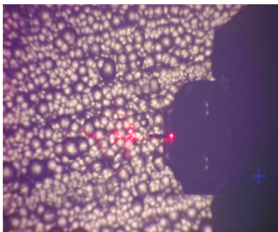
B-2 AFM video optical view of pyrolytic graphite sample. This enables users to visually locate a surface feature for AFM scanning.
