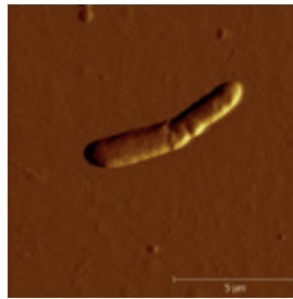
Image of an E. coli cell measured with the Dunk and Scan probe holder.
