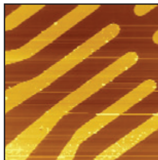
10 x 10 \mu\text{m} image of silicon sample with gold pattern. At the left is a topography image and at the right is a conductive AFM image. Two of the "fingers" on the test pattern are grounded and show contrast in the conductive AFM image.
