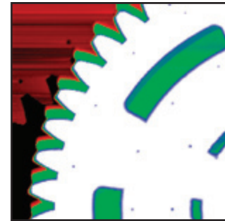
40 x 40 \mu\text{m} image of a gear fabricated with MEMS.
