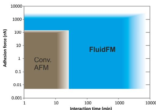
FluidFM extends accessible cell–substrate interaction time and interaction force by orders of magnitude, allowing experiments not feasible with conventional AFM methods to be performed.
