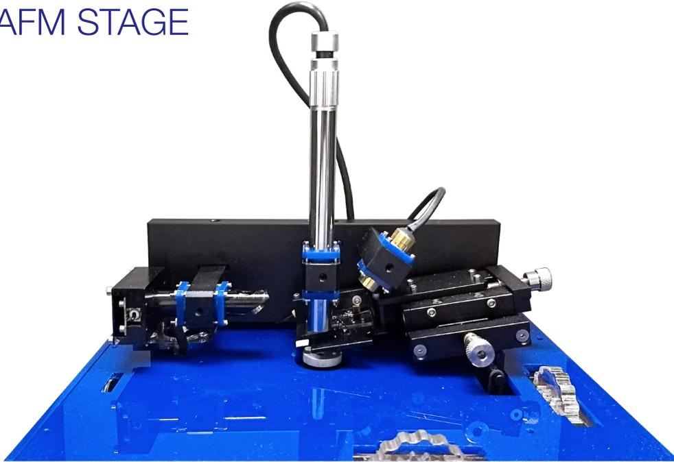
The **B-AFM** stage has an open design which makes exchanging samples and probes a straightforward process. Adjustments to the camera, photodetector, probe, and sample are all easily facilitated with the **B-AFM**. Students are able to see all of the components in action, allowing fast and simple operational and theoretical training.
