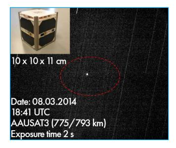
Fig. 2 shows a frame taken from a cube sat using an sCMOS camera (Zyla-5.5-CL10 from Andor Technology) with an exposure time of 2 secs in continuous tracking mode.
