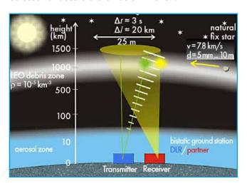
The general concept is depicted in Fig. 1. Space debris objects are first recognized by passive optical means using solar illumination. Afterwards, they are illuminated by an intense, highly repetitive, ns-pulsed, 532 nm time-of-flight (TOF) illumination laser.
