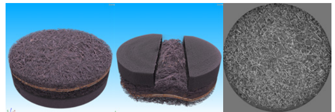
Fig. 1 Tomographic investigation of MEA assembly of PEM fuel cell. The diameter of the GDL fibres is approximately 10 \mu\text{m} . The experiment was performed at micro focus X-ray CT scanner using a high resolution detector based on sCMOS Andor Neo with an effective pixel size of 1.6 \mu\text{m} . The exposure time was 20 s per image. 1000 angular projections over 360° were recorded in 6 hours. Top and bottom view of the sample (on the left and in the middle). Single tomographic slice (on the right)
