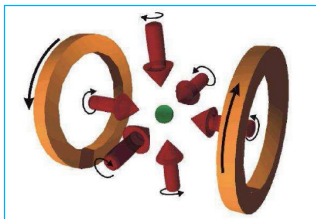
Figure 1 Schematic of a magneto-optical trap. Six laser beams (in red) cool the atomic cloud in all directions. A magnetic field, created by the circular coils, provides a position dependant force, keeping the atoms trapped.
