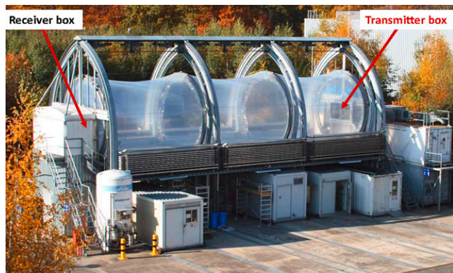
Fig. 2: The Atmosphere Simulation Chamber SAPHIR is a tool for the quantitative experimental investigation of tropospheric chemistry under natural conditions. Design features: double-wall Teflon foil cylinder, 5 m diameter and 20 m length, 270 m 3 volume. The optical path of the BBCEAS instruments runs along the central axis of the chamber.
