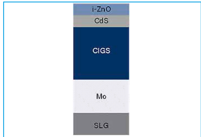
Fig. 2: Thin film sample consisting of a 50 nm thin ZnO layer, a 50 nm CdS layer, a 1.5 \mu\text{m} CIGS layer, and an approx. 400 nm thin Mo layer deposited on a soda lime glass (SLG) sample
