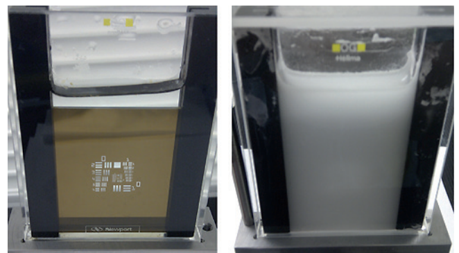
Figure 2: Resolution Target in a glass cell filled with water (left) and Resolution target in a glass cell filled with a suspension of water and polystyrene particles (right)
