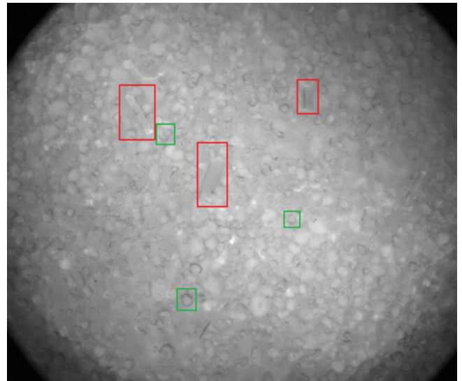
Fig. 13: Phosphors on a warm-white LED.
