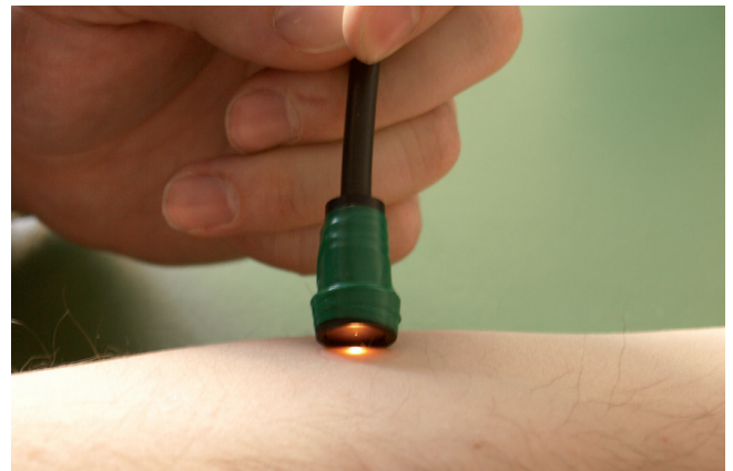
Figure 2: Determination of optical skin parameters and fluorescence with a reflecting measuring head.
