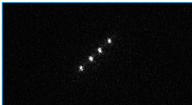
Figure 2: Fluorescence from a string of four calcium ions. The exposure time was 300 ms and the EM-gain was set to 3500. The distance between neighboring ions is about 10 \mu\text{s}
