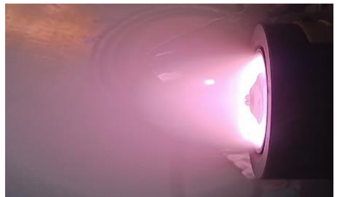
Figure 2: Hall Thruster in operation with argon as propellant [2]
