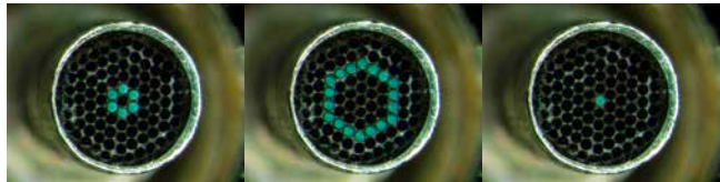
Figure 3: Fiber bundle for measuring the backscattered light (reflectance) dependent on the distance from the illumination.
