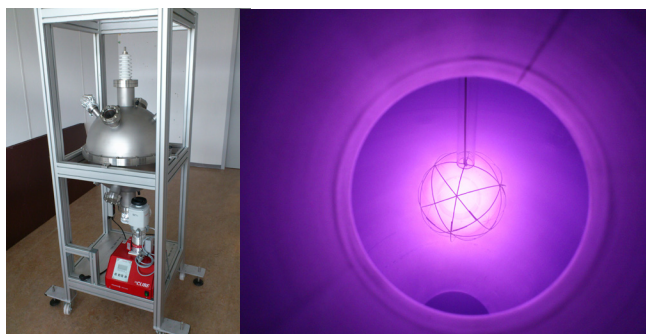
Figure 9 - The left picture shows the exterior of the fusor (before the voltage power supply and diagnostics were installed). The right picture shows the interior during operation.
