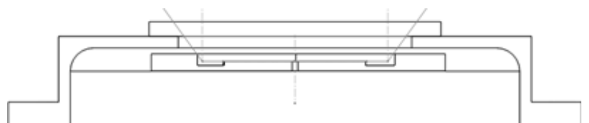
Figure 7: ‘Direct mount’ front end of Marana 4.2B-11, yielding f/\# 0.7 and 72^\circ Cone Angle. Discuss custom mounting flanges with Andor’s CSR Service.
